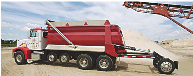
Trailing axle allows 25-ton payloads on a nimble straight truck in Hawaii. The bed's elliptical floor and wider sidewalls at the tailgate make for an easy, clean-dumping truck.
