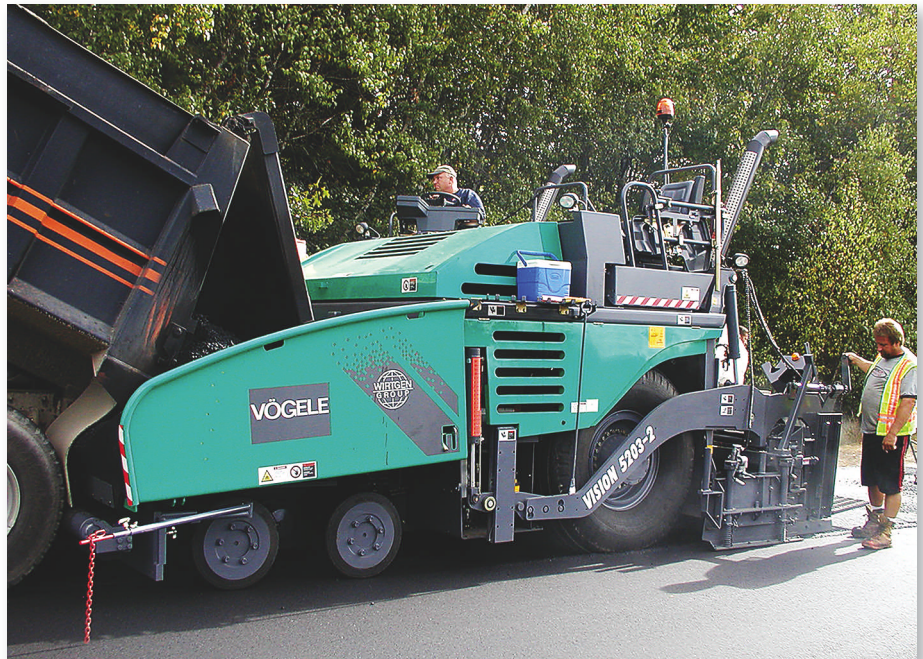
Vision series swing-out operator's stations and sliding consoles provide all-around visibility without the operator having to move around.
