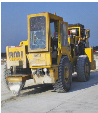
The shoe attached to the front of the steel beam vibrates at just \frac{1}{2} to \frac{3}{4} of an inch in amplitude, so only the concrete is broken.
